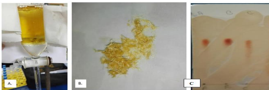
Figure 2 A: extraction of Kojic acid ; B: Kojic acid Crystals C: Kojic acid on TLC plate. Thin Layer Chromatography (TLC)
