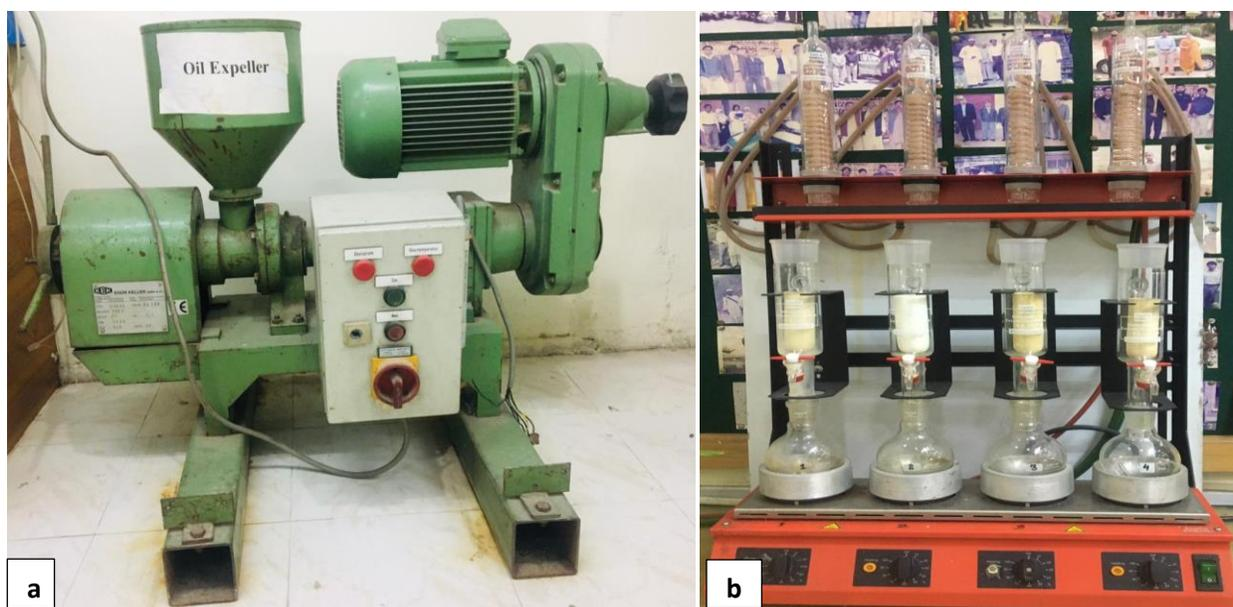
**Figure 3(a) Mechanical oil extractor (b) Soxhlet Apparatus**
