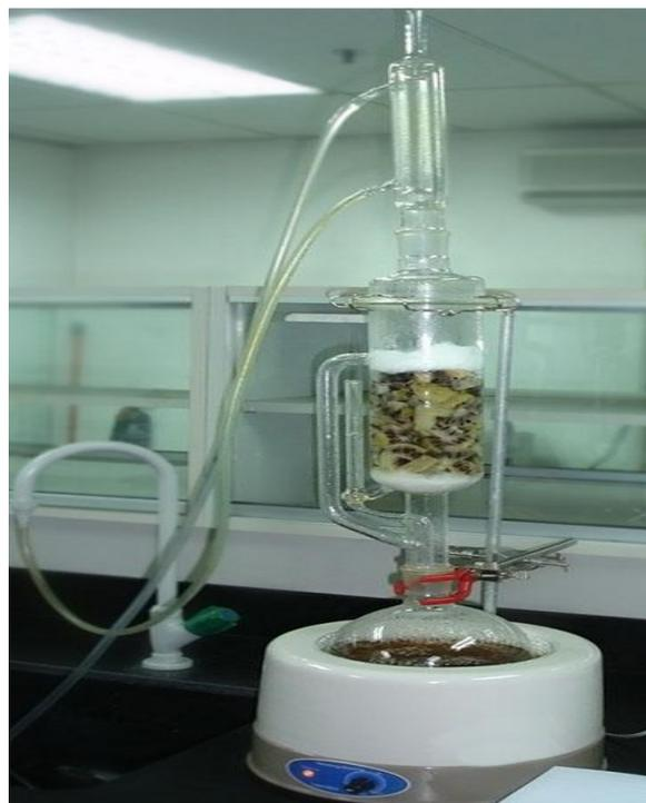
**Figure 1:** Soxhlet Apparatus
